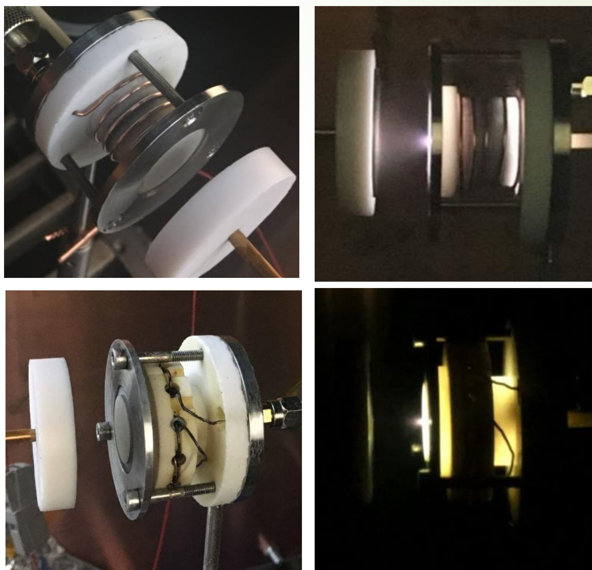
FIGURE 6. A biased electrode is placed 12mm in front of the cathode orifice for electron extraction
